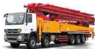
Mobile Concrete Pump 5
