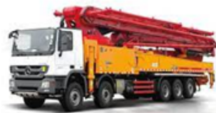
Mobile Concrete Pump 2
