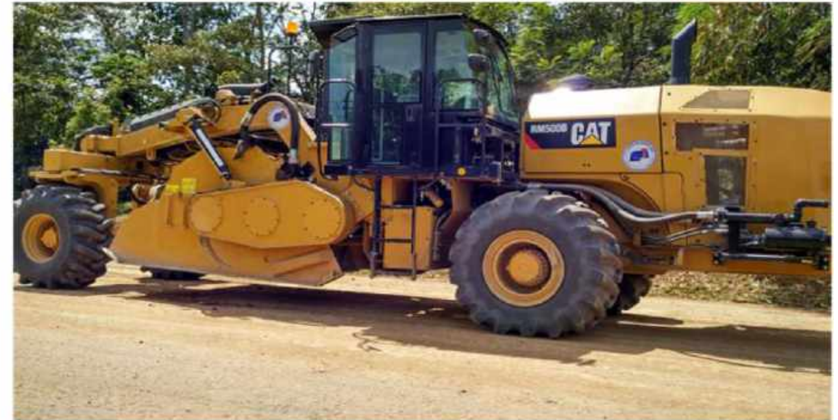
Soil Cement Stabilization (SCS)
